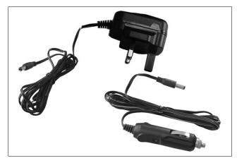
A 3 amp fuse is fitted into the cigarette lighter plug adaptor, accessed by unscrewing the two halves of the adaptor. Take care not to loose the spring when unscrewing this cap.
